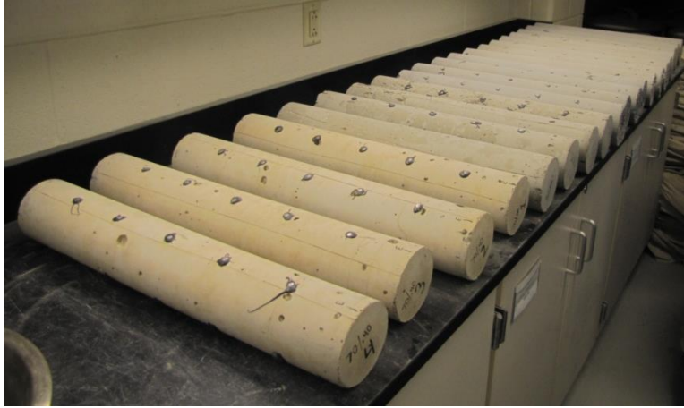
Figure 1: Shrinkage Specimens with DEMEC Strain Measurement Points
